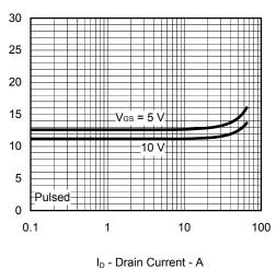
DRAIN TO SOURCE ON-STATE RESISTANCE vs.
