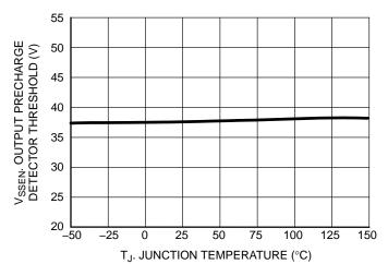
Figure 26. Output Precharge Detector Threshold vs. Junction Temperature
