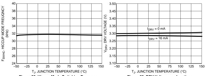
Figure 22. Hiccup Mode Switching Frequency vs. Junction Temperature
