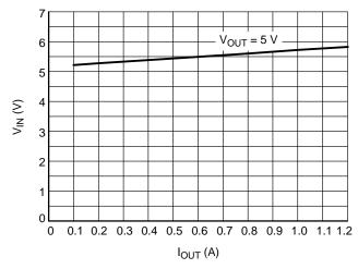
Figure 33. Minimum Input Voltage vs. Output Current
