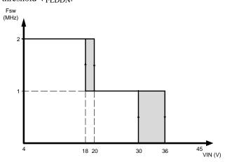
Figure 27. NCV890131 Switching Frequency Reduction at High Input Voltage
