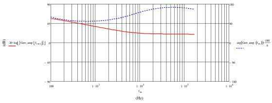
Figure 37. Bode Plot of the OTA Compensator
