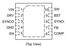
Figure 3. Pin Connections
