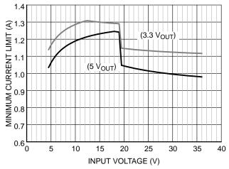
Figure 28. NCV890131 Load Current Capability with 4.7 µH Inductor
