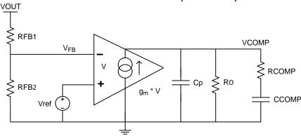
Figure 34. Feedback Compensator Network Model
