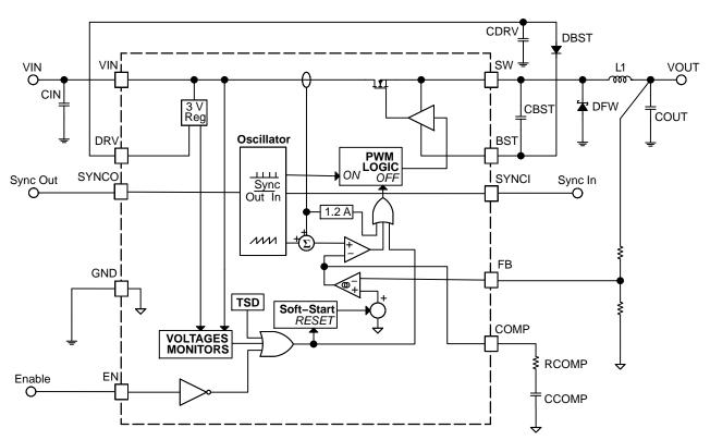
Figure 2. NCV890131 Block Diagram
