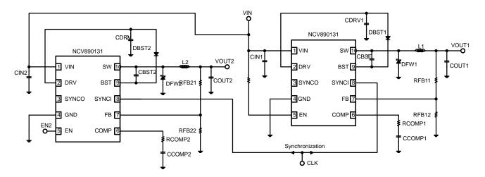
Figure 30. Both NCV890131s Synchronized to External Clock #1 Enabled by Battery
