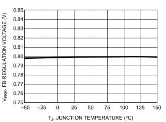
Figure 9. FB Regulation Voltage vs. Junction Temperature
