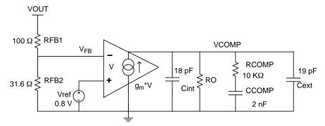
Figure 36. Example of the Feedback Compensation Network
