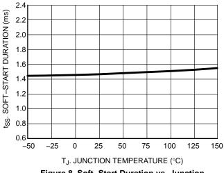
Figure 8. Soft-Start Duration vs. Junction Temperature
