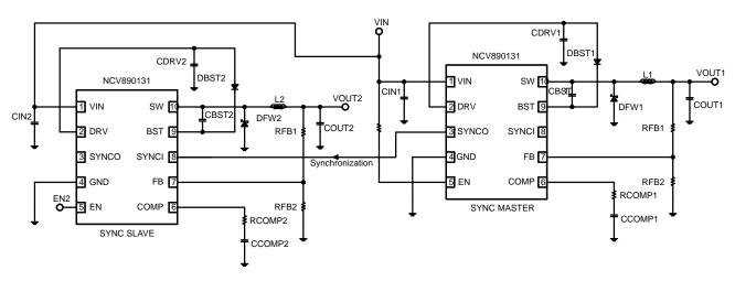
Figure 29. NCV890131s Synchronized to Each Other Master Enabled by Battery
