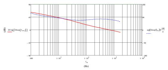
Figure 38. Bode Plot of the Total Loop
