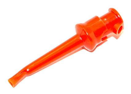
• The BU-P3925 is a standard DIY Plunger clip. It can be installed to wire up to 18 AWG with a jacket as large as  $\phi$  .09" (2.3 mm).
