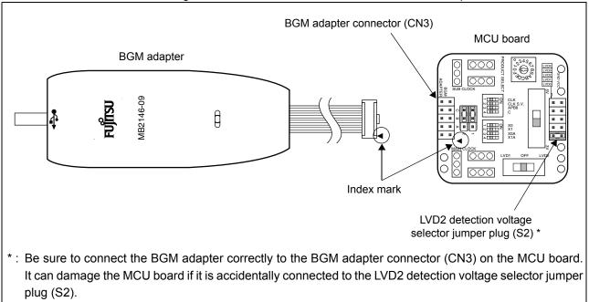
Figure 3-2. Connection of MCU Board and BGM Adapter
