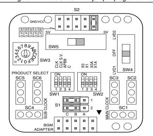
Figure 4-1. The switch and jumper plug on a MCU board
