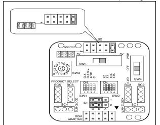
Figure 4-3. Positions of Switches and Jumper Plugs on the MCU Board
