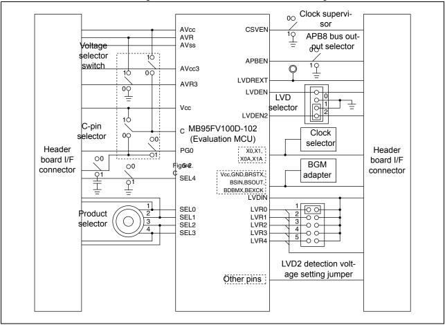
Figure 5-1. MCU Board Functional Block Diagram
