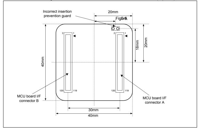
Figure 5-4. Recommended Dimensions of the Header Board (Top view)
