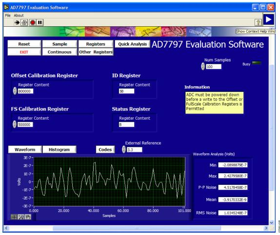
Figure 5. AD7797 Evaluation Software Other Registers Window
