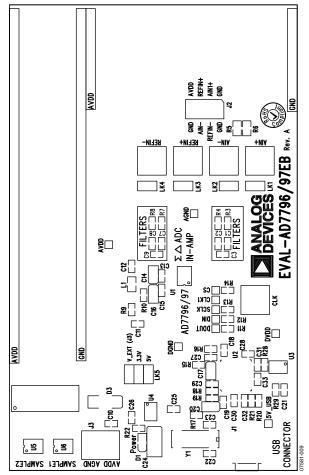
Figure 9. AD7797 Evaluation Board Component Layout Diagram
