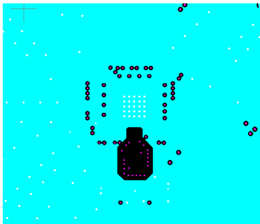
Figure 11.8. Bottom Layer Ground Flooded (Layer 3)
