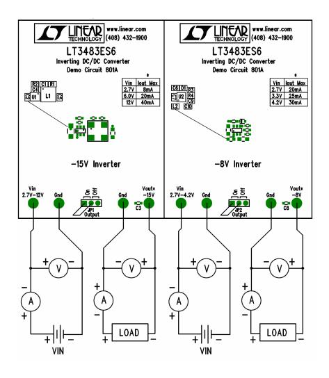
Figure 1. Proper Measurement Equipment Setup
