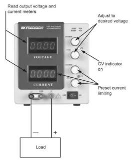
Figure 4 - Typical Constant Voltage Operation
