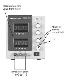
Figure 5 - Setting Current Limit
