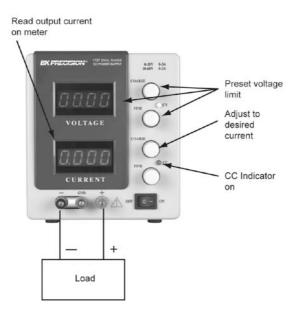
Figure 6 - Typical Constant Current Operation
