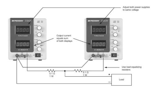
Figure 9 - Connecting Two Power Supplies in Parallel
