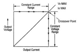
Figure 7 - Constant Voltage/Constant Current Characteristic
