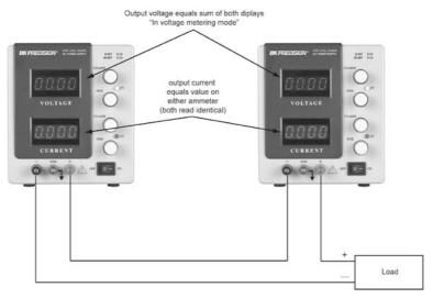
Figure 8 - Connecting Two Power Supplies in Series
