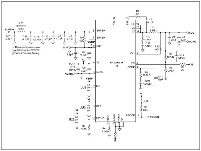
Figure 1. MAX20003 EV Kit Schematic
