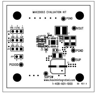
Figure 2. MAX20003 EV Kit Component Placement Guide—Component Side
