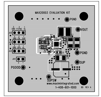
Figure 3. MAX20003 EV Kit PCB Layout—Component Side
