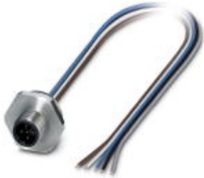
Sensor/actuator flush-type plug, 5-pos., M12, A-coded, front/screw mounting with M20 x 1.5 thread, with 0.5 m TPE litz wire, 5 x 0.34 mm 2 , high-grade steel version
