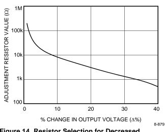
Figure 14. Resistor Selection for Decreased Output Voltage
