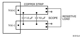
Note: Use a 1.0  $\mu$ F ceramic capacitor and a 10  $\mu$ F aluminum or tantalum capacitor. Scope measurement should be made using a BNC socket. Position the load between 51 mm and 76 mm (2 in. and 3 in.) from the module.
