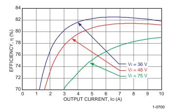
Figure 3. Typical Converter Efficiency vs. Output Current at Room Temperature
