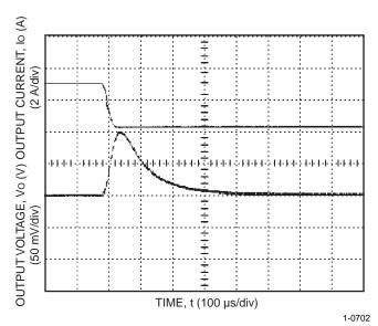
Note: Tested with a 10  $\mu F$  aluminum and a 1.0  $\mu F$  ceramic capacitor across the load.
