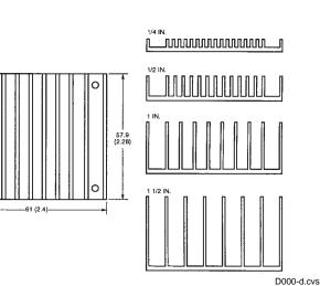
Figure 23. Transverse Heat Sink
