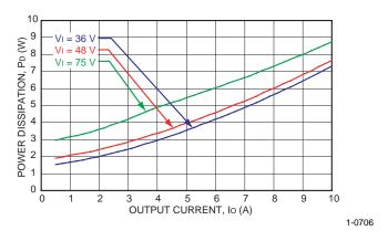
Figure 18. Power Dissipation vs. Output Current
