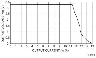
Figure 2. Typical Output Characteristics at Room Temperature
