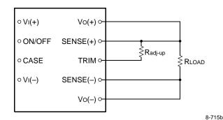
Figure 15. Circuit Configuration to Increase Output Voltage
