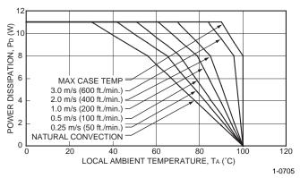
Figure 19. Forced Convection Power Derating with No Heat Sink; Either Orientation
