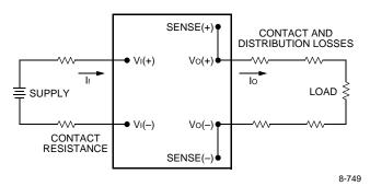
Note: All measurements are taken at the module terminals. When socketing, place Kelvin connections at module terminals to avoid measurement errors due to socket contact resistance.
