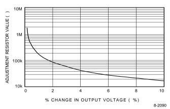
Figure 16. Resistor Selection for Increased Output Voltage
