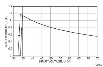
Figure 1. Typical Input Characteristics at Room Temperature
