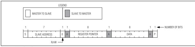
Figure 4. Write-Byte Format
