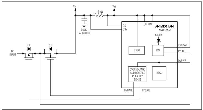
Figure 8. Overvoltage and Reverse Polarity Protection
