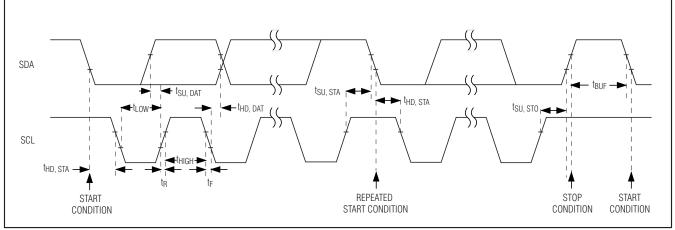
Figure 2. 2-Wire Serial Interface Timing Detail
