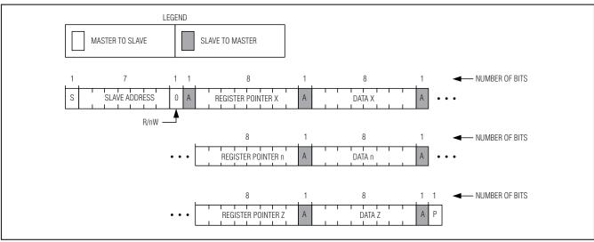
Figure 5. Multiple Bytes Register-Data Pair Format
