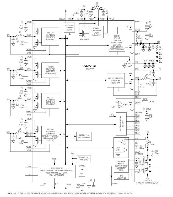
Figure 1. Typical Application Circuit and Function Diagram
