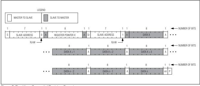
Figure 7. Read from Sequential Registers Format
